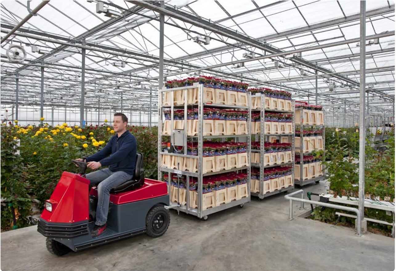
The 1500 is a compact sit-on electric tow tractor with a towing capacity of 2,000 kg and a low
